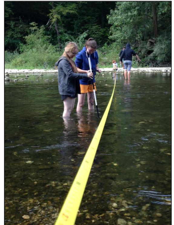
Fig. 1: Students measuring river depth and flow velocity. Source: Eder, S. (2015).
